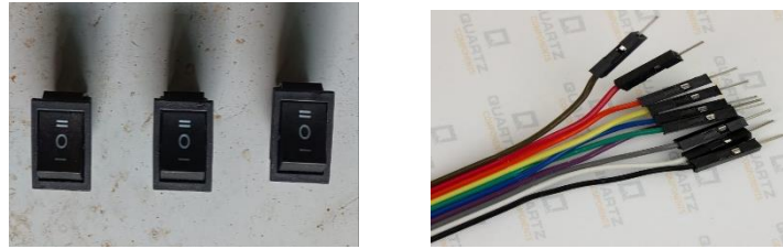
Photograph 3: The DPDT switch and Connecting Wires
