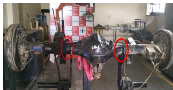
Fig. 5 Mounting of strain gauges on the axle housing to measure contact stresses
