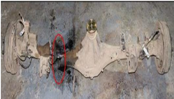
Fig. 2 Fracture of the rear axle housing at the left side
