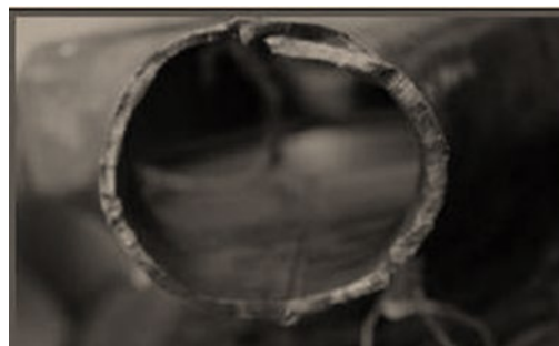
Fig. 3 Rear axle housing broken piece
