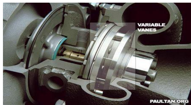
Fig.4.1 Cut-section of Variable Geometry Turbocharger (when the vanes are fully open).[2]
