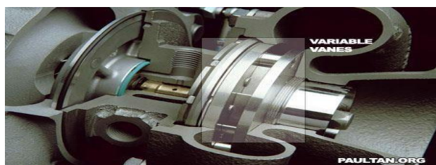
Fig.3.1 Cut-section of Variable Geometry Turbocharger (when the vanes are almost closed). [2]
