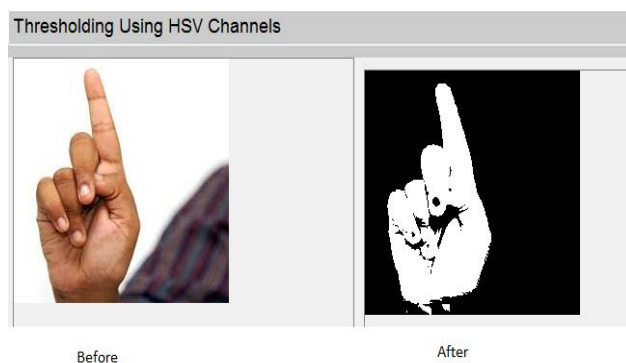
Fig. 8. Thresholding using HSV
