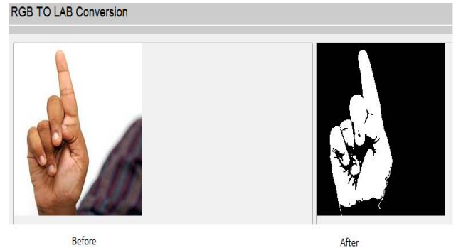
Fig. 9. Thresholding using LAB
